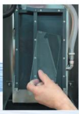
The unique sensing chamber design alows easy access to the controls and wetted components. The lamp/receiver unit is simply lifted and placed onto the convenient door rack. For any routine cleaning, the flow plate can be wiped in place or removed.
