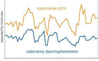
The HydroSense 2410 correlates well against laboratory methods and is ideal for process trending and continuous on-line monitoring.
