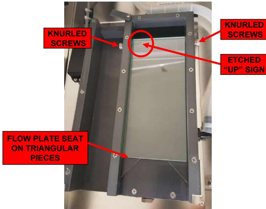
**Figure 2 – FLOW PLATE SECURE AGAINST TRAY**
