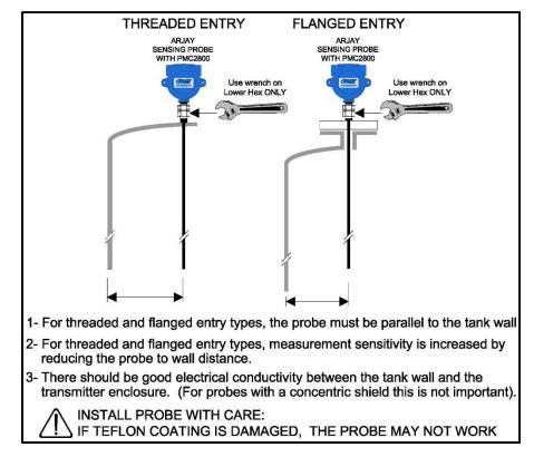
Figure 2 – Probe Installation
