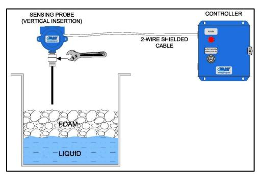
Figure 1 – Typical Installation
