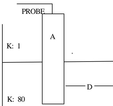
If the tank is filled with water ( $K = 80$ ), it displaces air ( $K = 1$ ), and we have a dramatic change in capacitance which is utilized in the electronics to activate a relay or transmit a signal proportional to the amount of water in the tank. The electronics allow for tuning of the system so that the operator can activate a relay at any point or measure between a wide choice of spans.
