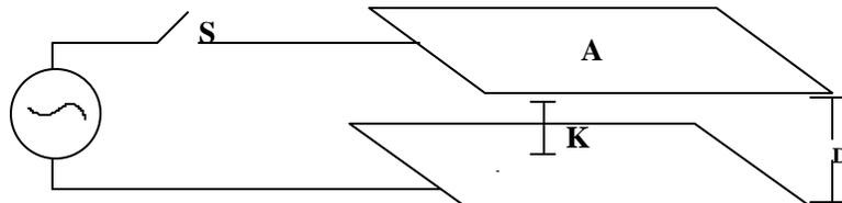
The formula for current flow through a capacitor with an alternating voltage applied is  $I=V2 FK/A/D$ . K is defined as the dielectric of material or ability to store electrons.
