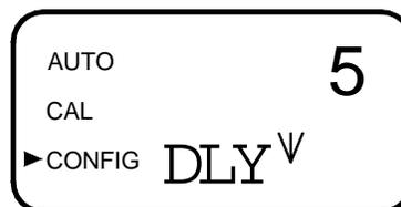
The current selected number of seconds will be shown. Select the desired delay off time for this alarm using the **▲** and **▼** buttons. Once the desired delay time has been set, press the **↵** button to accept it. After the settings for alarm 1 have been completed, prompts will allow for the set up of the information on alarm #2.
