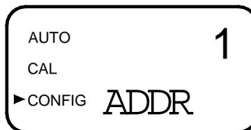
To enable the Modbus mode, select **ASCII** or **RTU**. Refer to the Modbus Manual, if this option was purchased, for more information.
