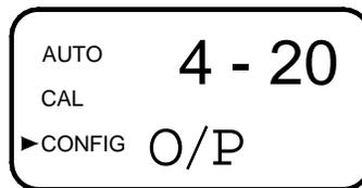
If the 4-20 mA output was turned on, prompts to set the lower (**LOLM**) and upper (**UPLM**) ppm limits corresponding to the 4 mA and 20 mA output levels will be displayed. The first prompt will be the ppm limit assigned to the 4 mA output level:
