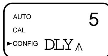
The current selected number of seconds will be shown. Select the desired number of seconds for the "delay on" time for this alarm using the **▲** and **▼** buttons. Once the desired delay time has been set, press the **↵** button to accept it.
