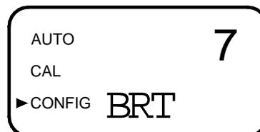
Change the brightness by pressing the ▲ or ▼ button. When the desired brightness has been selected, press the ↵ button.
