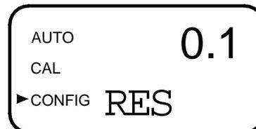
Change the resolution by pressing the ▲ or ▼ button. When the desired digit resolution has been selected, press the ↵ button.
